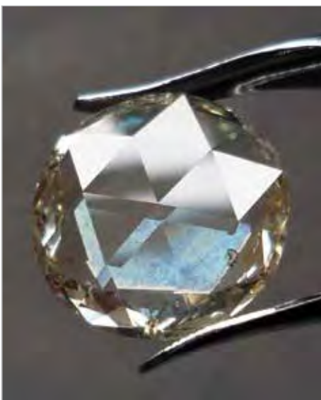
6: 'Thin' rose-cut diamond, 15 mm diameter, 7.19 ct.
